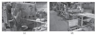
Figure 2.2 Phases of the manufacturing process of GFRP bars: (a) raw glass fibers in rovings; (b) glass fibers drawn through a resin bath for impregnation and a metal die; (c) solid bar emerging from the curing oven; (d) cured bar ready to be cut at the desired length.
