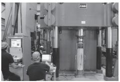
(a) MTS test frame with data-acquisition system
