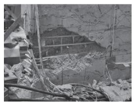
(b) Concrete crushing causing failure
