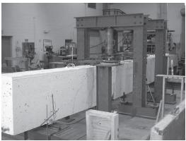
(a) Immediately prior to failure with marked-up cracks
