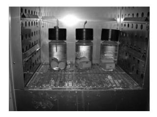
Figure 3.18 Water absorption test.
