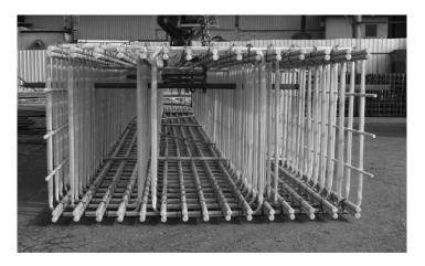
Figure 1.12 GFRP reinforcement cage for soft-eye construction at a manufacturing plant (Angri, Italy).
