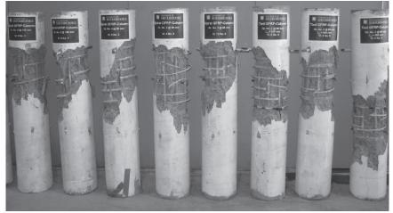
(c) Column specimens after failure
