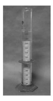
Figure 3.1 Measurement of the cross-sectional area of an FRP bar by the Archimedes principle.
