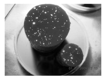
Figure 3.19 Voids due to the presence of hollow glass fibers.
