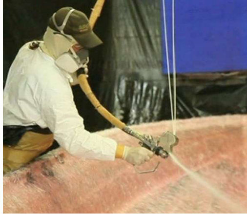
Figure 4: Laying up a fiberglass boat with a chopper gun (Fibers and resin are sprayed on)
