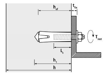
h = thickness of member $h_1 = depth of drill hole$
