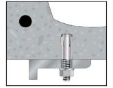
5. Installed SA in precast prestressed hollow core slab
