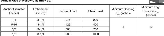
All values are based on mortar shear strength of 40 psi or greater. 1
