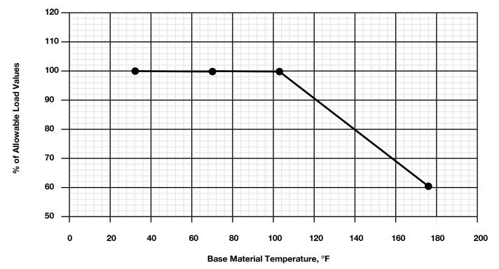
1 Short term temperature loading only for temperatures greater than 122 °F. Short term elevated temperatures are those that occur over brief intervals, e.g., as a result of diurnal cycling. Long term temperatures are roughly constant over significant periods of time. 2 Published allowable tension and shear loads shall be reduced by the reduction percentage listed above.
