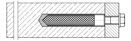
Pre-positioned installation with subsequently injected fischer filling disc (annular gap filled with mortar)
