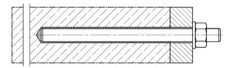
Push through installation (annular gap filled with mortar)
