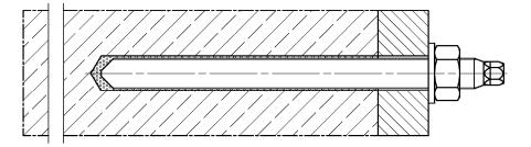
Pre-positioned installation with subsequently injected fischer filling disc (annular gap filled with mortar)
