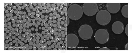
SEM analysis confirmed that there was **no sign of deterioration** in the GFRP coupons. Glass fibers were intact **without loss of any cross-sectional areas**. Fibers were surrounded by the resin matrix and **no gap nor sign indicating the loss of bond between resin and fibers**, was observed.
