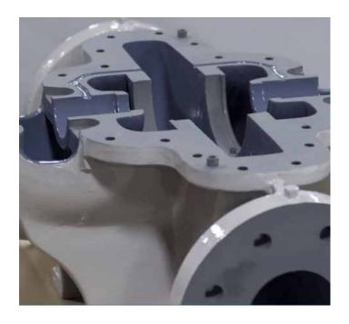
Belzona 5821 is a multi-purpose brush or spray applied coating that provides outstanding protection from the effects of salt, water, acids, alkalis, alcohols and hydrocarbons.
