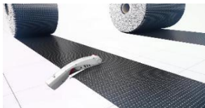
Cutting carbon fiber cloth
