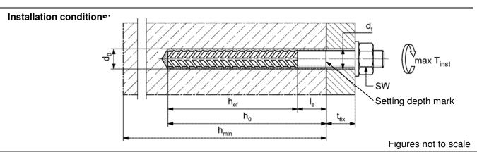
fischer injection system FIS EM Plus for use in uncoated liquid-tight sealing systems made of concrete (FD  $\!\!/$  FDE concrete) in SFH facilities
