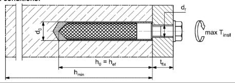
fischer injection system FIS EM Plus for use in uncoated liquid-tight sealing systems made of concrete (FD / FDE concrete) in SFH facilities
