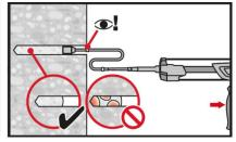
$\label{eq:hef} \begin{array}{l} \text{Injection} \text{ method for drill hole depth} \\ h_{\text{ef}} > 250 \text{mm}. \end{array}$
