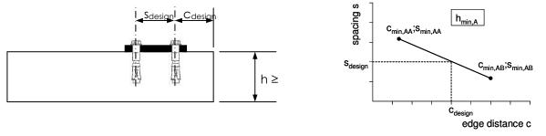
FIGURE 4—Example of allowable interpolation of minimum edge distance and minimum spacing
