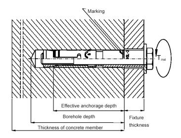
FIGURE 3—CORRECT INSTALLATION OF HSL-3 (BOLT VERSION SHOWN)
