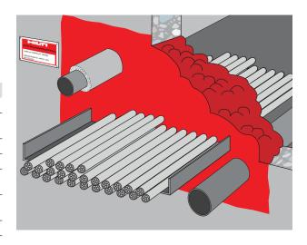
Use a suitable tool to create an opening (screwdriver, drill bit etc.). Push the cable or pipe through and then seal the remaining opening carefully with CP 620.
