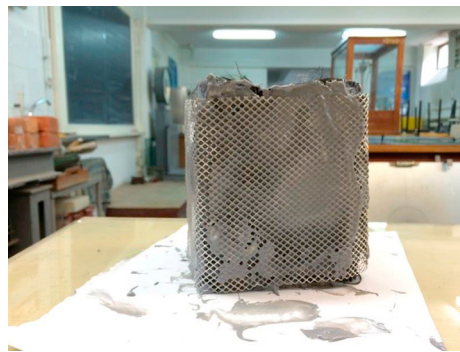
Fig. 6. Sandwich of bricks reinforced with carbon and aluminium
