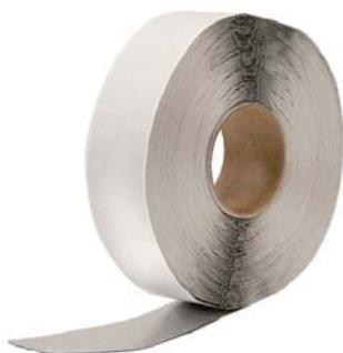
A self-adhesive tape based on rubber butyl reinforced on one side with aluminum foil. The tape forms a high vapour barrier and is waterproof, so it can be used for a wide range of construction applications.
