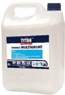
Multigrunt is a concentrated primer based on two types of acrylic dispersions that strengthen the substrate, leveling the absorbency and increasing the adhesion of screeds, adhesives, plasters, and interior and exterior paints. It penetrates the substrate, strengthens the surfaces, binds the loose particles and limits the water absorption of the substrate.
