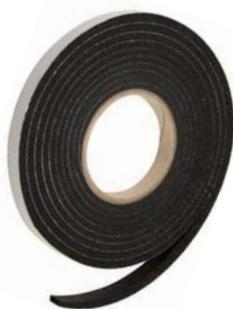
A self-adhesive, impregnated tape based on polyurethane foam with open cells. It does not contain plasticizers. The tape is packed in rolls compressed to approx. 15–20% of the target thickness, and expands slowly in the gap when released from the roll. Depending on the requirements, there are several types of tapes with different water resistance index: BG1, BG2 and DB.
