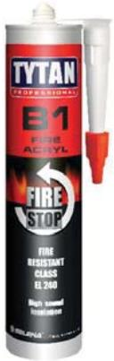
High specification formulation designed to prevent the spread of fire, smoke and gases through openings in fire rated walls and floors, specifically linear movement joints and openings for building service penetrations. B1 Fire Acryl expands when it is subjected to fire and closes openings around penetrations when any combustible or low temperature melting materials have burnt away.
