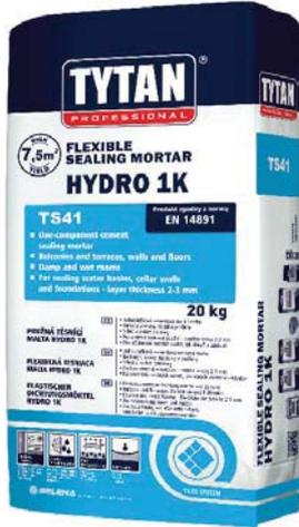
Sealing Mortar Hydro 1K is a one-component product suitable for making light, medium, heavy moisture and water insulation. It creates a tight, flexible and seamless coat to bridge substrate cracks and provide a permanent sealing for corners, expansion joints and sanitary pipe passes in connection with special sealing tapes and flanges of the Tytan water insulation system.
