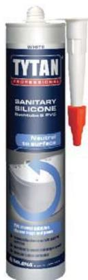
Fast curing silicone containing fungicides that protect joints against fungi and mildew. It has a perfect adhesion, especially to acrylic bathtubs and PVC. With its neutral cure formula, it is virtually odourless and does not cause corrosion. Once cured, it creates a non-shrink and elastic joint.
