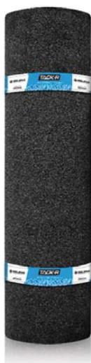
Tack-R Green S40 is a torch-on foundation bituminous membrane with polyester reinforcement. It is modified with SBS. It is confirmed by FLL certificate to be resistant to root penetration.
