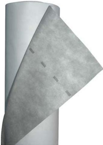
Three-layer vapor-permeable roof membrane. Made of two layers of polypropylene nonwoven and special functional film which ensures high vapor permeability and water tightness of the underlay. Owing to its high vapor permeability, it can be applied directly on insulation and consequently a venting slot is not required between the membrane and the thermal insulation.
