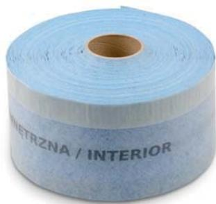
Window Tape Interior provides an additional insulating layer between the wall and frame of windows or doors, thus protecting the joints from absorbing the moisture from the room. The tape consists of a high quality vapour barrier membrane, which guarantees the optimum value of  $S_d \geq 50$  m, coated on both sides with non-woven polypropylene.
