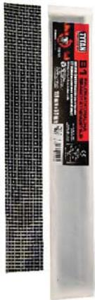
B1 Fire Wrap is designed to maintain the fire resistance of fire separating walls and floors when these are breached by continuous plastic pipes or metal pipes with combustible insulation and may be used in gypsum, masonry or concrete walls and concrete floors. Each pipe wrap consists of a graphite based reactive intumescent strip which reacts to heat and closes the opening left by the softening plastic pipe or pipe insulation in fire.
