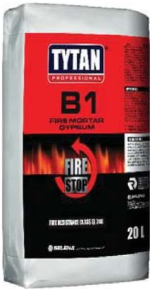
B1 Fire Mortar Gypsum is a dry white powder consisting of inorganic compounds and perlite. When mixed with water the compounds form a highly thermally insulating fire seal to prevent the spread of fire and smoke through openings in fire rated walls and floors, including openings formed to accommodate building service penetrations.
