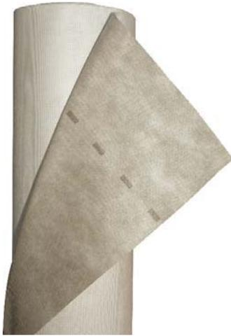
Three-layer vapor-permeable roof membrane. Made of two layers of polypropylene nonwoven and special functional polyethylene film which ensures high vapor permeability and water tightness of the underlay. Owing to its high vapor permeability, it can be applied directly on insulation and consequently a venting slot is not required between the membrane and the thermal insulation.
