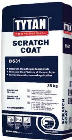
Scratch Coat is a cement based mortar applied directly onto the substrate before the application of finish layer of Tytan Building System. It is recommended for the mineral substrate preparation which will receive cement-lime plaster machine or manually applied. It improves the plaster adhesion to walls and ceilings, and levels the substrate absorption.
