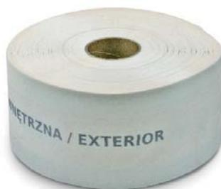
Window Tape Exterior provides an additional insulating layer between the wall and frame of windows or doors, preventing the joints from absorbing the rain and wind and improving the overall insulation parameters. The tape consists of a high quality vapour permeable membrane, which guarantees the optimum value of  $S_d \leq 0,05$  m, coated on both sides with nonwoven polypropylene.
