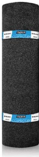
Tack-R SF20 S25 is a self-adhesive foundation bituminous membrane with polyester reinforcement. Modified with SBS and additives improving adhesion parameters.
