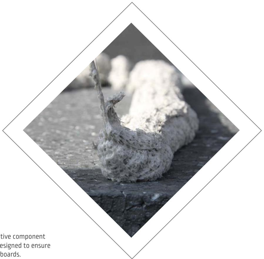
Fast adhesive for ETICS is a unique and innovative component of Tytan FGS (Fast Grab System). It has been designed to ensure an easy and convenient bonding of Insulation boards.
