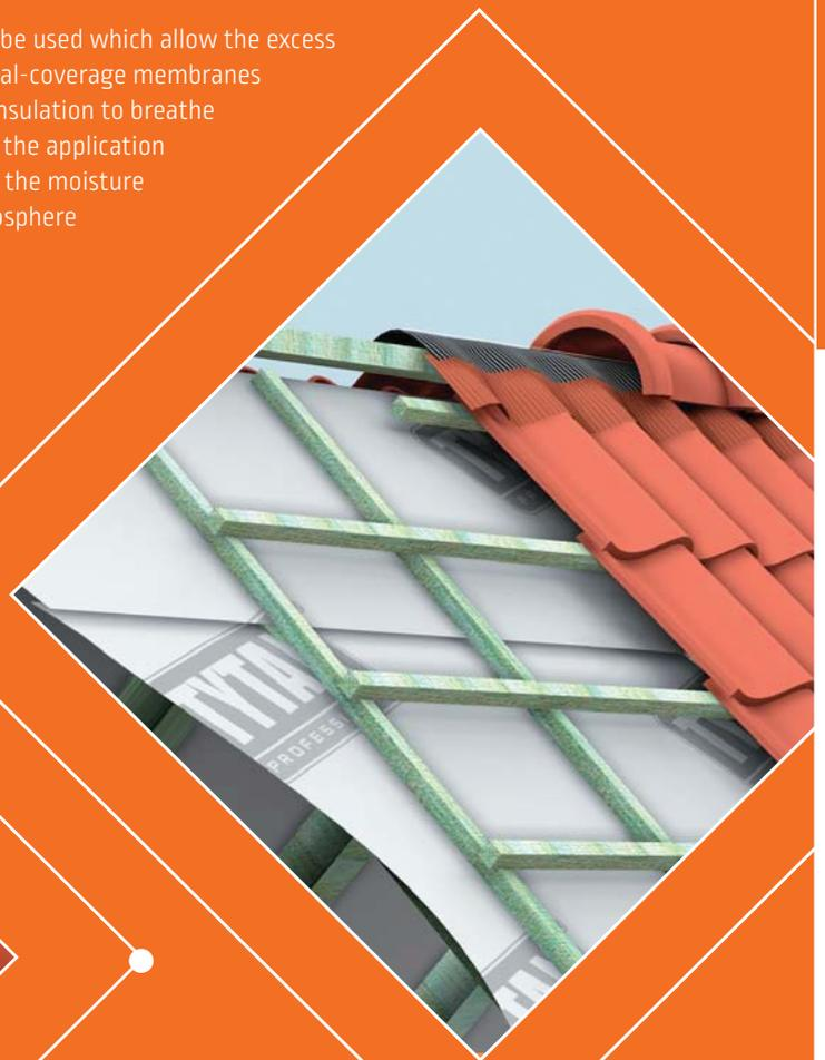
A ridge is the crucial element in the process of ventilation of the roof cover. In order to ensure its proper progress, we use special, highly vapour-permeable ridge tapes. They protect the inside of the roof cover against dust, nesting birds and precipitation and, at the same time, transfer damp air outside.
