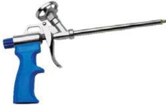
A new generation gun applicator which guarantees increased foam yield. The valve is opened mechanically by contact with the can and is not dependent on the pressure inside the can.
