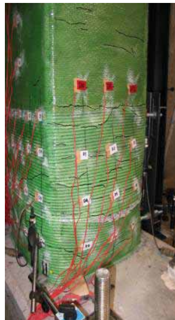
(b) Column retrofitted with PET sheet
