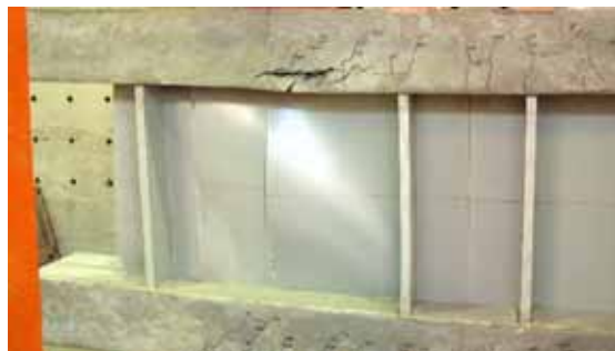
Figure 9 Boxed-sectioned prestressed concrete girder bridge with GFRP web panel
