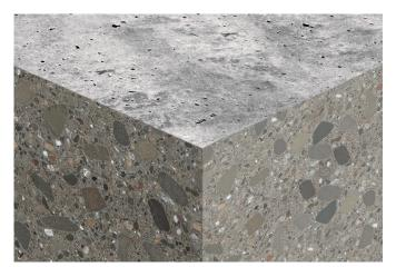
LI/LIP concrete in general is a type of concrete with optimised resistance against penetration by water polluting substances. LIP concrete is a liquid impermeable concrete after penetration testing. LI/LIP concrete is designed so as to be considered liquid impermeable.
