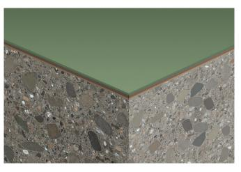
If the WRL surface is created by applying a coating to the concrete, then the coating alone is responsible for sealing against water polluting substances. fischer has developed a system in which the seal against water polluting substances is retained, even if holes are drilled into the coated concrete.
