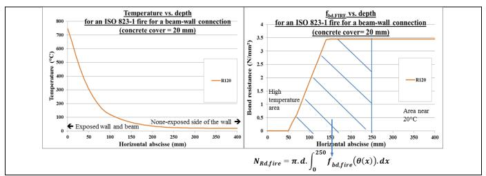
Figure 8 : General example of the calculation of the design load resistance by integration of  $f_{\mbox{\scriptsize bd}}$
