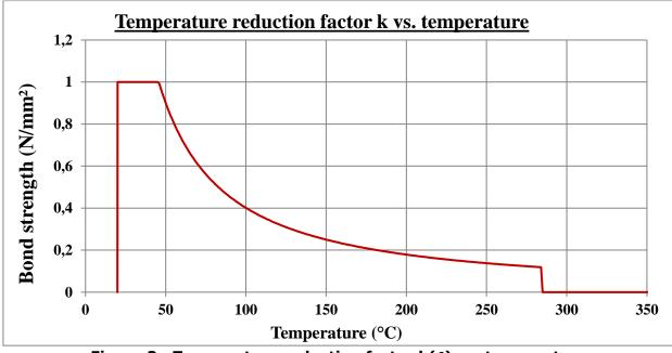
Figure 3 : Temperature reduction factor  $k(\theta)$  vs. temperature
